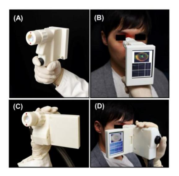
This shows photographs of the power grip style (A-B) and camcorder style designs (C-D) of the prototype OCT scanner. Both devices acquire 3D OCT images of the retina. Credit: *Biomedical Optics Express*
