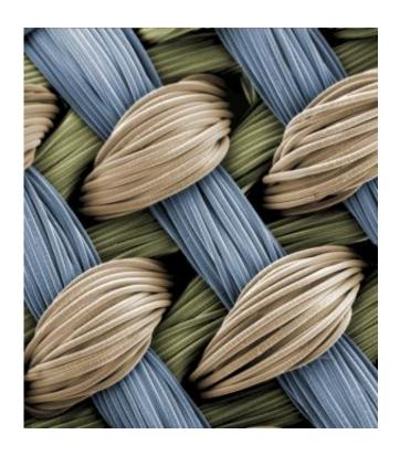
Tiny interwoven fibers make up the three-dimensional fabric "scaffold" into which a strong, pliable hydrogel is integrated and injected with stem cells, forming a framework for growing cartilage. This image appears on the cover of the Dec. 17, 2013, issue of *Advanced Functional Materials*. Credit: Frank Moutos and Farshid Guilak
