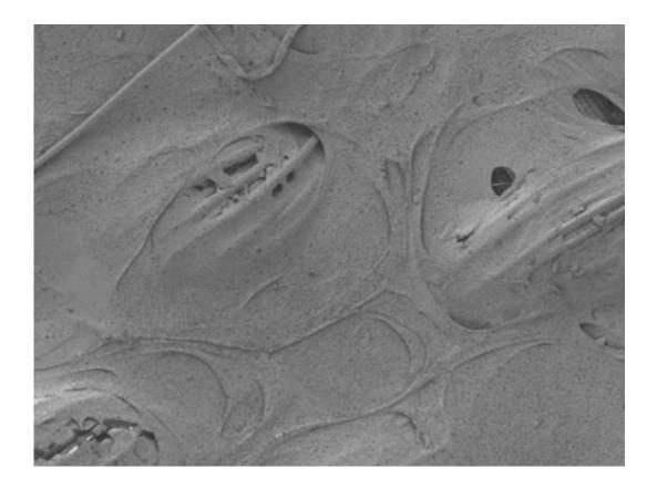
This is a closer look at the scaffolding integrated with Xuanhe Zhao's hydrogel. The composite material, formed through a process comparable to pouring concrete over a steel framework, may be a serviceable synthetic replacement for the load-bearing cartilage found between bones. Credit: I-Chien Liao, Frank Moutos, Brad Estes
