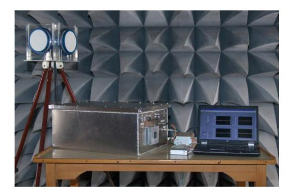
Tools for defending against electromagnetic attack (right to left): an antenna set (on tripod) for sensing the environment, a RF measuring device for conditioning the signals and a computer that calculates the relevant data. Credit: Fraunhofer INT
