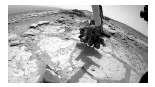
An image from the curiosity rover's front hazard-avoidance camera shows the rover drilling into its second rock target, "Cumberland."Credit: NASA/JPL-Caltech
