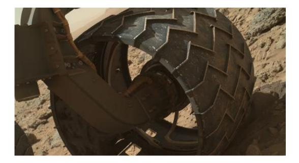
The left-front wheel of NASA's Curiosity Mars rover shows dents and holes in this image taken during the 469th Martian day, or sol, of the rover's work on
