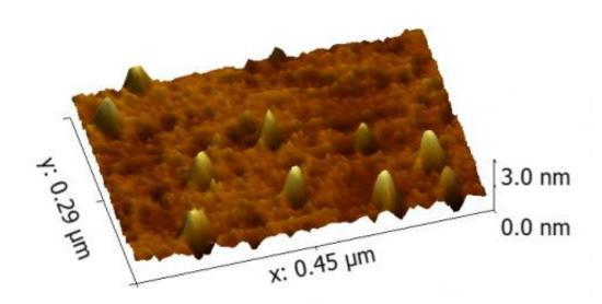
Piles of zero-dimensional carbon nanotubes appear as gold "mountains" on a substrate by atomic force microscopy. The nanotube mountains are only a few nanometers high – or nearly a billion times smaller than an inch. Credit: University of Pittsburgh Swanson School of Engineering
