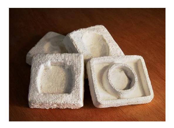
Biomass packaging material created using technology developed by ARS, collaborators, and Ecovative can be made to custom fit a wide variety of products. Credit: Ecovative.
