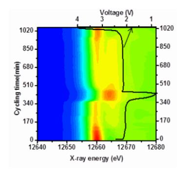
Normalized XANES spectra of Li/Se cell during cycling. Black line is the battery voltage profile.
