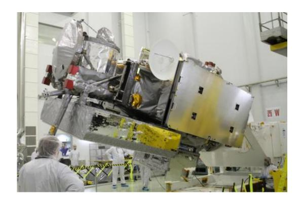
Following arrival in a cleanroom at the Tanegashima Space Center in Japan, the Global Precipitation Measurement (GPM) core observatory was attached to a custom-designed satellite mount which allowed the NASA team on-site to perform preliminary inspections and evaluations of the spacecraft. Credit: NASA/Michael Starobin
