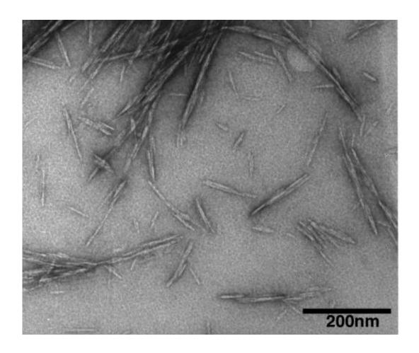
This transmission electron microscope image shows cellulose nanocrystals, tiny structures that give trees and plants their high strength, light weight and resilience. The nanocrystals might be used to create a new class of biomaterials that would have a wide range of applications. Credit: Purdue Life Sciences Microscopy Center
