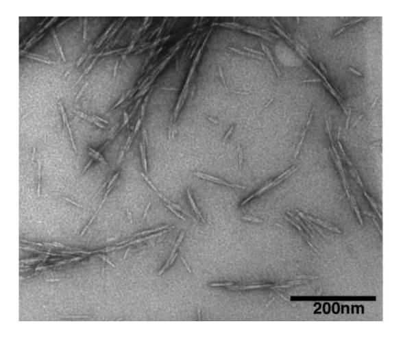
This transmission electron microscope image shows cellulose nanocrystals, tiny structures that give trees and plants their high strength, light weight and resilience. The nanocrystals might be used to create a new class of biomaterials that would have a wide range of applications. Credit: Purdue Life Sciences Microscopy Center
