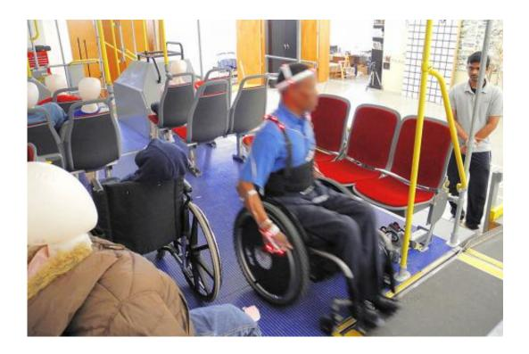
A volunteer outfitted with motion sensors navigates a full-scale replica of a public bus. The University at Buffalo's Center for Inclusive Design and Environmental Access (IDeA Center) is studying how to improve the design of buses by analyzing what works and what doesn't with current models. Credit: UB IDeA Center
