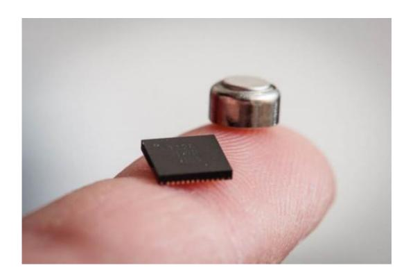
Imec, Holst Centre and Wicentric introduce today their integrated ultralow power Bluetooth Smart radio solution for a range of smart applications. With a power consumption up to five times lower than stateof-the-art radios and an extremely small memory footprint, this radio solution, integrating imec and Holst Centre's 2.4GHz ultra-low power radio and Wicentric's exactLE product line of Bluetooth® Smart
