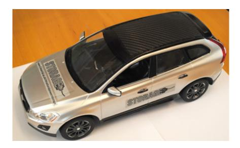
To combine energy storage with mechanical strength is a unique compromise. In the model above, the car roof has been replaced by a structural battery. Credit: Emilia Lundgren
