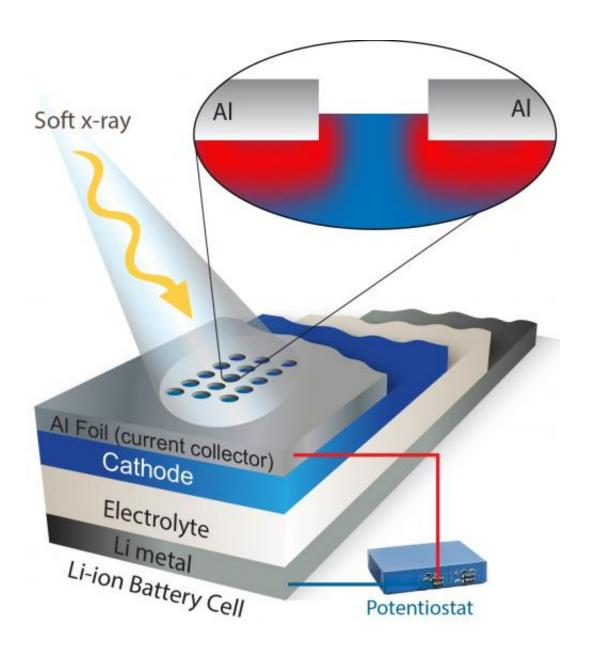
This schematic depicts a new spectroscopy technique that offers a never-beforeseen look at how electrodes function. Windows etched into a foil covering allow
