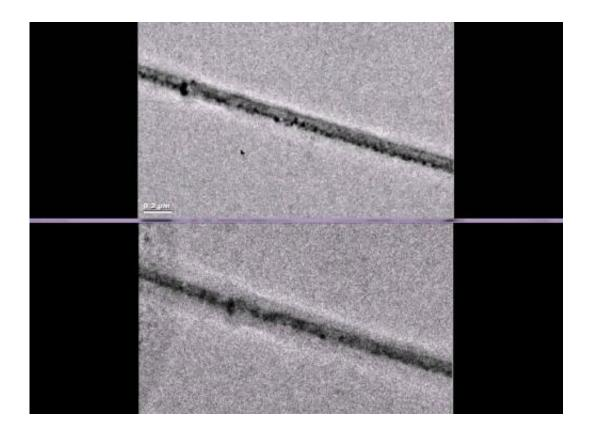
Researchers can now view a battery at work in the high magnification world of transmission electron microscopy. Liquid battery electrolytes makes this view of an uncharged electrode (top) and a charged electrode (bottom) a bit fuzzy. Credit: Gu et al, *Nano Letters* 2013
