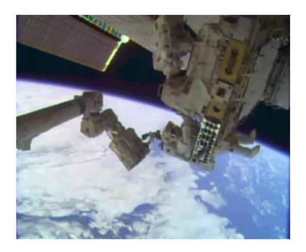
In this image taken from video provided by NASA, astronauts Rick Mastracchio, top, and Michael Hopkins work to repair an external cooling line on the International Space Station on Tuesday, Dec. 24, 2013, 260 miles above Earth. The external cooling line—one of two—shut down Dec. 11. The six-man crew had to turn off all nonessential equipment, including experiments. (AP Photo/NASA)
