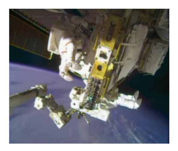
In this image taken from video provided by NASA, astronauts Rick Mastracchio, top, and Michael Hopkins work to repair an external cooling line on the International Space Station on Tuesday, Dec. 24, 2013, 260 miles above Earth. The external cooling line—one of two—shut down Dec. 11. The six-man crew had to turn off all nonessential equipment, including experiments. (AP Photo/NASA)
