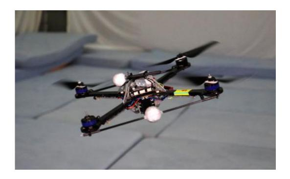
Even after loss of a propeller, a quadrocopter remains airborne thanks to a new control algorithm. Credit: Mark Mueller / ETH Zurich
