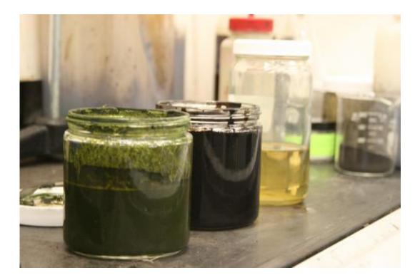
(L-R): Algae slurry; biocrude oil; and, with further processing, refined biocrude which contains mostly the makings of gasoline and diesel fuel Credit: Photo by PNNL
