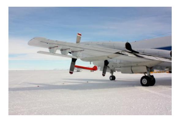
A MCoRDS's underwing radar antenna arrays mounted beneath the wing of NASA's P-3 aircraft at McMurdo Station's airfield is shown. MCoRDS uses arrays beneath the wings and fuselage of the plane, giving a total of 15 antennas that can send and receive signals used to map polar ice and bedrock. Credit: NASA/George Hale
