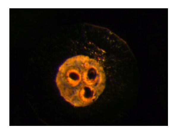
This shows thin slices of basalt with a diameter of just a fraction of a millimeter were subjected to high pressure in a diamond anvil cell. This sample has been molten and subsequently probed with X-rays three times. Credit: Chrystèle Sanloup, University of Edinburgh
