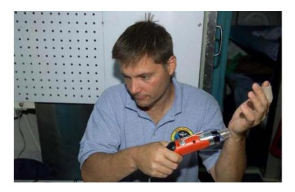
There are many ideas for investigating bone health in astronauts. Here, astronaut Doug Wheelock uses an Acoustic Vibration Bone Quality Measurement Device in 2004 during NEEMO 6, one of an underwater series of missions NASA ran to simulate space exploration. Credit: NASA
