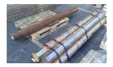
Large-scale manufacture of nanostructured steel shafts. Credit: Rolls Royce Plc.
