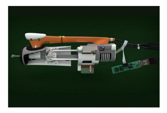
A carving tool designed by MIT Media Lab postdoc Amit Zoran, called FreeD, allows the user to control the carving process while aided by a computer guidance system that is preprogrammed with the desired three-dimensional shape. Credit: MIT
