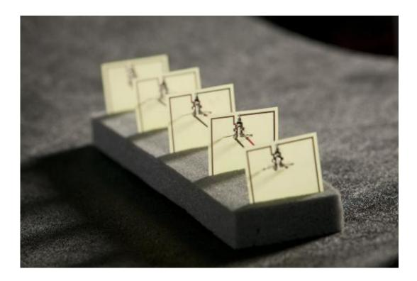
This five-cell metamaterial array developed at Duke University has a powerharvesting efficiency of 36.8 percen -- comparable to a solar cell. Credit: Duke University
