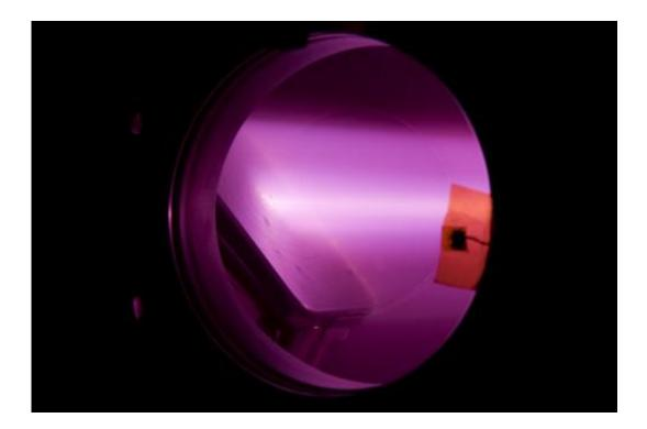
DIFFER's devices Pilot-PSI and Magnum-PSI can test materials under the hot, dense plasma conditions of future fusion reactors. Credit: DIFFER
