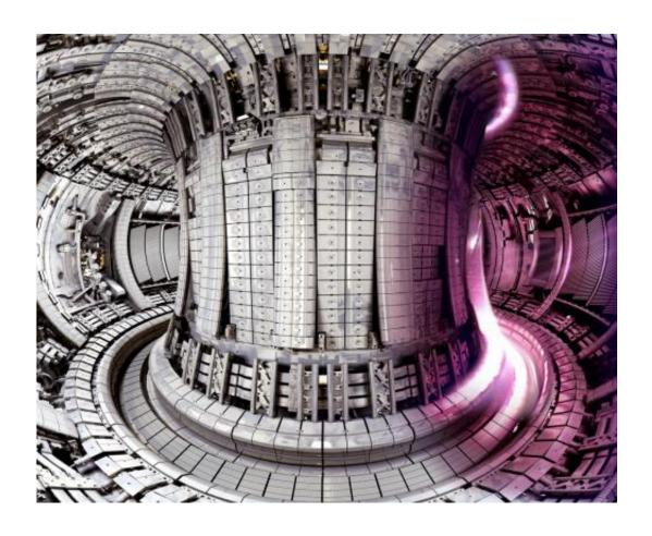
The European fusion reactor JET near Oxford was given a tungsten internal wall in 2010. Credit: CCFE / JET
