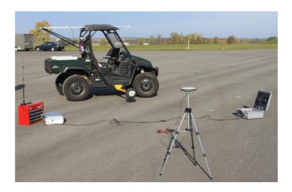
An experimental four wheel independently actuated, lightweight electric vehicle. Credit: Junmin Wang, Ohio State University
