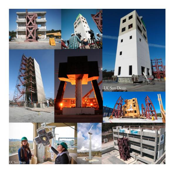
The NEES @ UCSD shake table has been used to test a wide variety of structures. Clockwise from center of top row: a five-story building equipped with non-structural components (two pictures), a soft-story wood frame building, a precast concrete structure, a wind turbine, interior of the five-story building's surgery suite, a seven-story building, a three-story masonry building and a bridge column (image at the center). Credit: Jacobs School of Engineering/UC San Diego
