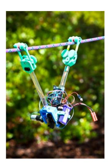
SkySweeper is V-shaped with a motor-driven "elbow" and its ends are equipped with clamps that open and close as necessary to move it down utility lines, searching for damage, inch by inch. Credit: Jacobs School of Engineering/UC San Diego
