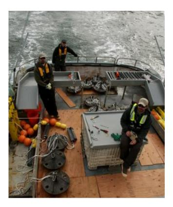
The PNNL crew heads out from the mouth of the Columbia River and into the ocean. The yellow receivers are attached to the round anchors and can detect fish up to 250 meters away. L-R: Scott Titzler, Ryan Harnish, Mike Hughes. Credit: Geoff McMichael/PNNL
