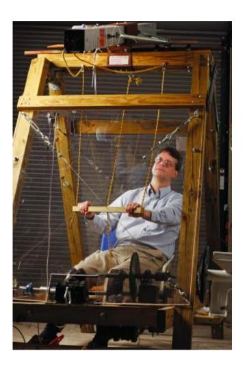
This is David Olinger, associate professor of mechanical engineering at Worcester Polytechnic Institute, with a rig that uses a rocking arm to translate the motion of wind-powered kite into rotary motion to spin an electric generator or power a device like a water pump. With an award from the National Science Foundation, Olinger is currently exploring the use of underwater kites to generate power from currents and tidal flows. Credit: Worcester Polytechnic
