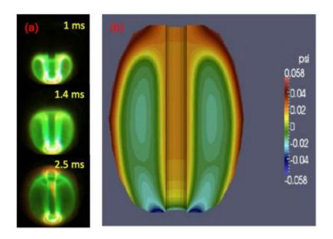
(a) This is a sequence of visible fast camera images of a CHI discharge inside NSTX. The top image shows the expansion of the CHI discharge one thousandth of a second after it is initiated. As shown in the third frame, within three thousandths of a second the plasma has fully filled the vessel; (b) the magnetic structure of a bubble in NSTX as simulated by the NIMROD code. Credit: Fatima Ebrahimi, Roger Raman, and Edwin Bick Hooper
