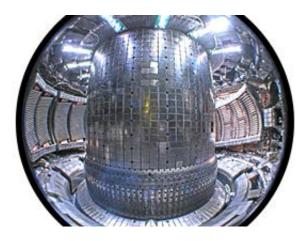
The tiled walls inside the Alcator C-Mod tokamak might say they've been scarred by sudden disruptions in the hydrogen fuel that periodically impacts them. MIT researchers are discovering ways to spread out the focused energy from these disruptions so that the vessel walls are not damaged. Credit: M. Garrett
