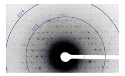
Image shows electron diffraction from lysozyme microcrystals prepared by Tamir Gonen's laboratory at HHMI's Janelia Farm Research Campus. Credit: Gonen Lab
