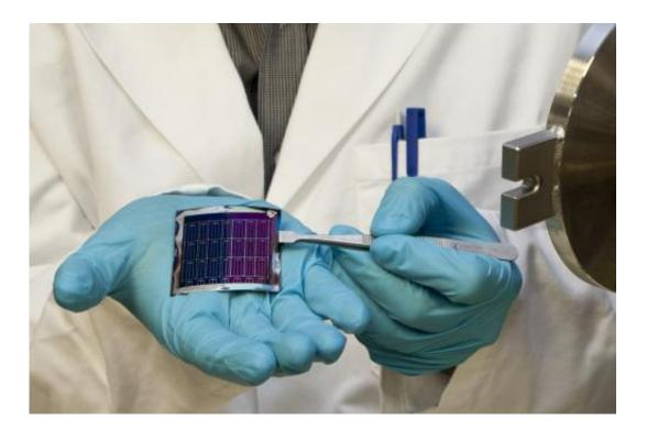
This shows high efficiency, flexible CIGS solar cells on polyimide film developed using a new process. Credit: Empa
