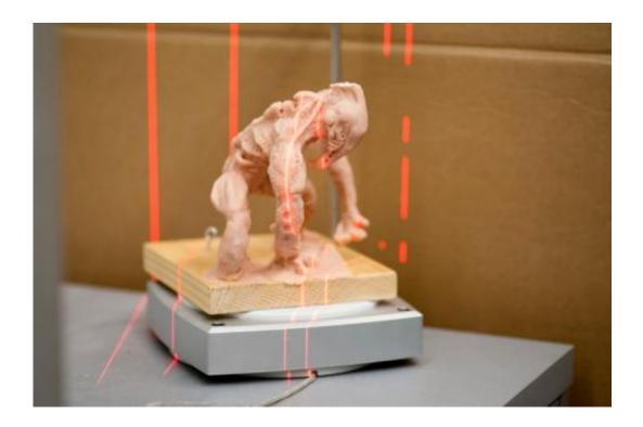
A clay model is analyzed by a laser scanner for reproduction.
