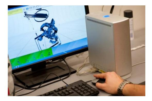
A computer displays a 3-D rendering of the clay model being analyzed by the laser scanner.
