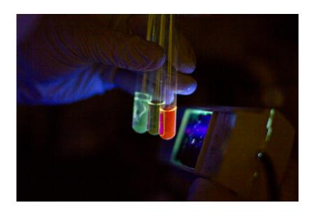
A researcher holds test tubes containing experimental molecules placed in a solution to demonstrate their unique optical properties, including the emission of photons of specific colors. The molecules are being tested to assess their potential as organic light emitters. Credit: Jessica Hochreiter/ASU
