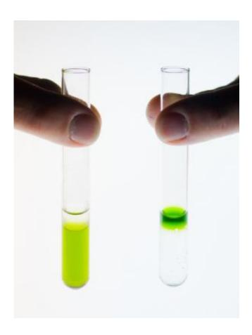
Special bacteria can turn biological waste into fuel by converting pigments in their cells into a type of biofuel called phytol—which separates out into the colorless top layer on the left.
