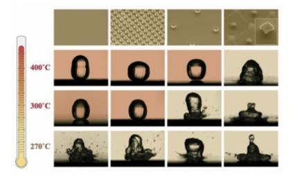
A micrograph showing water droplets landing on specially designed silicon surfaces (top images) at different temperatures. At higher temperatures, the droplets begin to exhibit a new behavior: instead of boiling, they bounce on a layer of vapor, never really wetting the surface.
