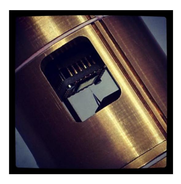
A section of a scanning probe microscope using the world's smallest SQUID (Superconducting Quantum Interference Device) created to date, probing a sample to measure its magnetic field. This novel instrument may help toward understanding superconductivity and gain insights into novel physics phenomena.
