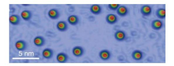
Three-dimensional topographic STM image of single Ho atoms adsorbed on Pt(111) at 4.4 K. Credit: *Nature* 503, 242–246 (14 November 2013) doi:10.1038/nature12759
