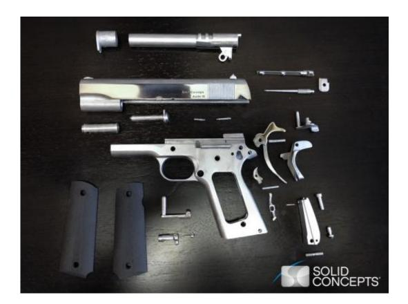
(Phys.org) —3D printing company Solid Concepts has <u>announced</u> that it has 3D printed the world's first metal gun—other guns printed using 3D printers have been made of plastic. Representatives for Solid Concepts say they created the gun to demonstrate how strong and accurate products made using 3D printing technology can be.
