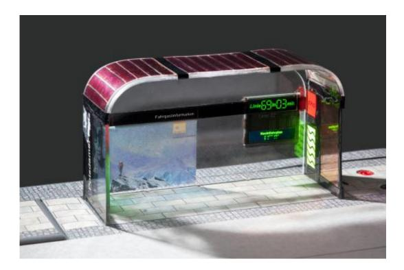
Organic light-emitting diodes (OLEDs) – here at the bus stop of the future – will soon come out of printing machines. Credit: © Fraunhofer IAP / Till Budde
