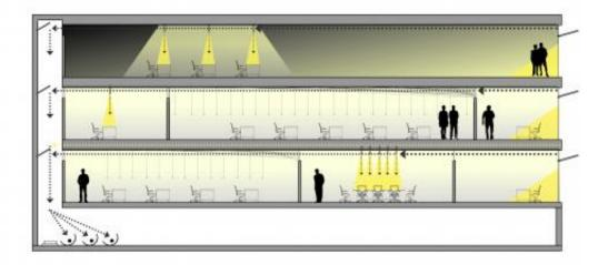
This diagram shows how the University of Cincinnati's SmartLight can direct sunlight from the outside of a building (far right) to the inner part of a building and to a centralized harvesting- and energy-storage hub (far left). Credit: Anton Harfmann, UC
