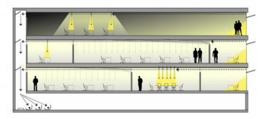
This diagram shows how the University of Cincinnati's SmartLight can direct sunlight from the outside of a building (far right) to the inner part of a building and to a centralized harvesting- and energy-storage hub (far left). Credit: Anton Harfmann, UC
