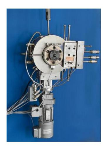
onBOX uses a sensor system to test the composition of plastics enriched with nanoparticles. The unit is mounted directly onto the mixing plant, and is able to monitor particle distribution. Credit: © Fraunhofer ICT
