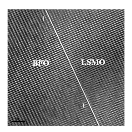
This high-resolution TEM micrograph shows BFO grown on a silicon substrate and aligned with an LSMO (lanthanum strontium manganese oxide) electrode.
