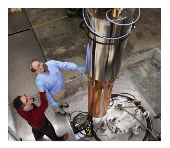
University of Washington physicists Leslie Rosenberg (right) and Gray Rybka examine the experiment package as it is positioned above the bore of a large superconducting magnet, two primary components of the detector being used in the Axion Dark Matter Experiment. The components were assembled in mid-October and lowered into the magnet bore (lower right) to begin the detector's commissioning phase. Credit: Mary Levin / University of Washington
