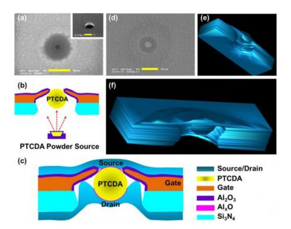
(a) SEM image of a nanopore with metal gate. Inset shows the tilt-angle view. (b) Deposition of a PTCDA nanoparticle in a nanopore, and (c) a nanoparticle located in a nanopore and sandwiched between electrodes. (d) SEM image of a nanoparticle in a nanopore. (e, f) Reconstructed 3D-TEM images of the nanoparticle inside the nanopore. Credit: Linh-Nam Nguyen, et al. ©2013 AIP Publishing LLC
