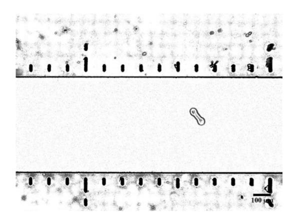
A slightly asymmetrical particle flows along the center of a microfluidic channel.
