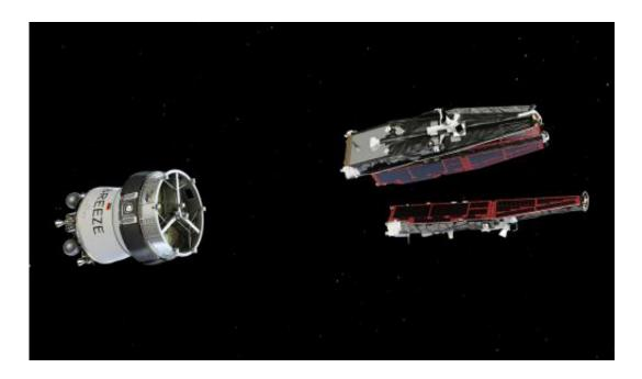
The three Swarm satellites are launched together on a single Rockot from Plesetsk, Russia. The satellites are placed on a Breeze-KM upper stage with a tailor-made dispenser for simultaneous separation. Credit: ESA/ATG Medialab
