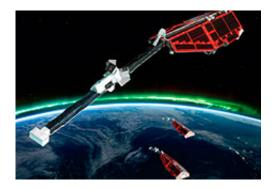
Two of the three identical Swarm satellites will orbit the Earth at a height of 450 kilometres, mapping the more subtle features of the Earth's magnetic field with more precision than ever before.
