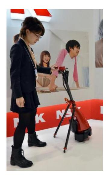
Japan's auto parts maker NSK demonstrates a cane style navigation 'LIGHBOT' robot for elderly and handicaped people, equipped with a laser rangefinder to avoid obstacles, at the annual Internatinal Robot Exhibition in Tokyo, on November 6, 2013
